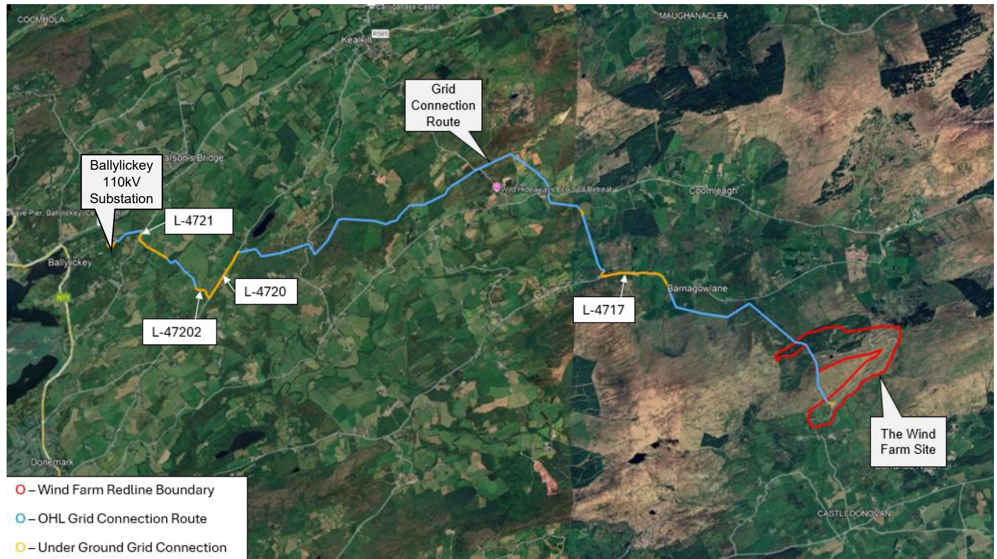
Figure 11.2: Grid Connection Route
